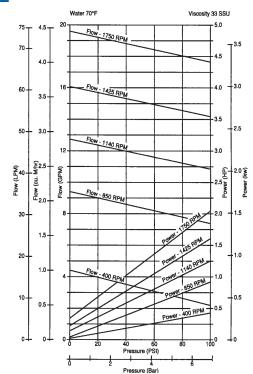
Notes: For continuous service: Plastic / Plastic gear combinations are limited to 50 psi. Metal / Plastic gear combinations are limited to 100 psi. Horsepower requirements increase for viscous fluids.
