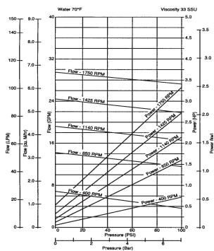
Notes: For continuous service: Plastic / Plastic gear combinations are limited to 50 psi. Metal / Plastic gear combinations are limited to 100 psi
