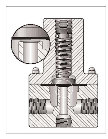
Diaphragm pressure relief valves are designed to protect chemical feed systems from over pressure damage caused by defective equipment or a blockage in the chemical feed line. Robust construction ensures reliability in the rigorous service of municipal and industrial applications. Materials of construction include PVC, 316 SS, and Hastalloy C®. Available in sizes 1/4" through 1 1/2".
